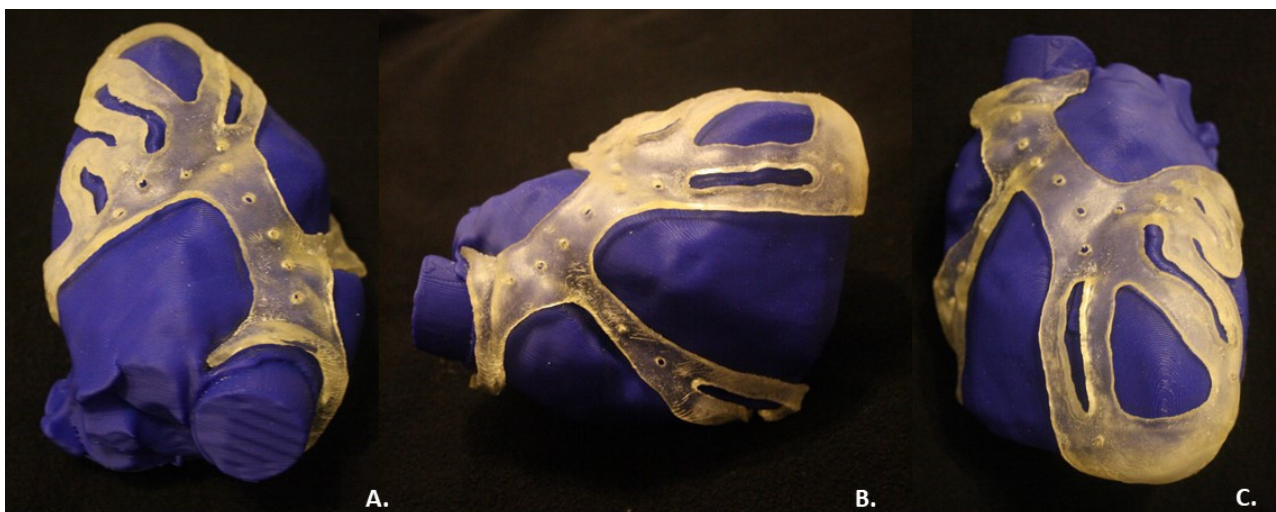
Figure 7. Fitting test of the surgical guide on the phantom heart: (A) Above view; (B) Right lateral view; (C) Frontal view.
