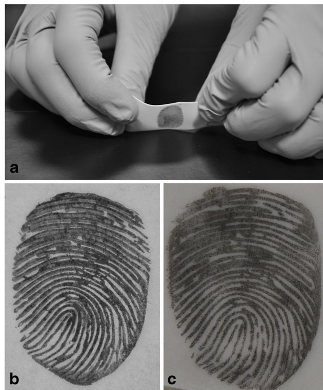
Fig. 1 Photographs of lifting fingerprints (These images were made using an artificial fingerprint to protect personally identifiable information (PII). The print was manufactured using computer aided design (CAD) software and fabricated with a 3D rapid prototyping printer. A cast was made of the resulting fake ‘finger’ using dental casting stone, and ballistics gelatin was poured into the cast to create an artificial finger. This gelatin finger was used to deposit sebaceous fingerprints for photographing and publishing purposes. More details of this process will be published elsewhere.). a Lifting the powdered latent fingerprint. b and c are side by side comparisons of resulting fingerprint lifts from a common tape pull using forensic tape ( b ) and the new adhesive swab lift ( c ). Note that ( c ) was originally a mirror image of ( b ); thus computer software was used to horizontally invert the image
