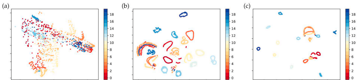
Fig. 1. Comparison of different dimensional reduction algorithms on Coil 20 dataset. Total 20 different labels are in the Coil 20 dataset, and we use the ground truth label to color each data points. (a) Feature size is reduced to dimension 2 by PCA. (b) Feature size is reduced to dimension 2 by t-SNE. (c) Feature size is reduced to dimension 2 by UMAP.
