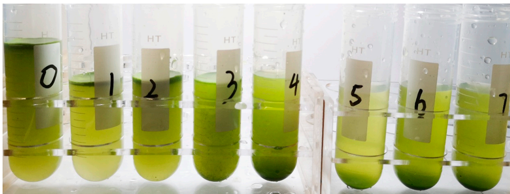
Figure 5. The settlement performances of WT cells in the water column after different static pressure treatments. The tubes from left to right were the samples pressurized by 0, 0.1, 0.2, 0.3, 0.4, 0.5, 0.6 and 0.7 MPa, respectively.
