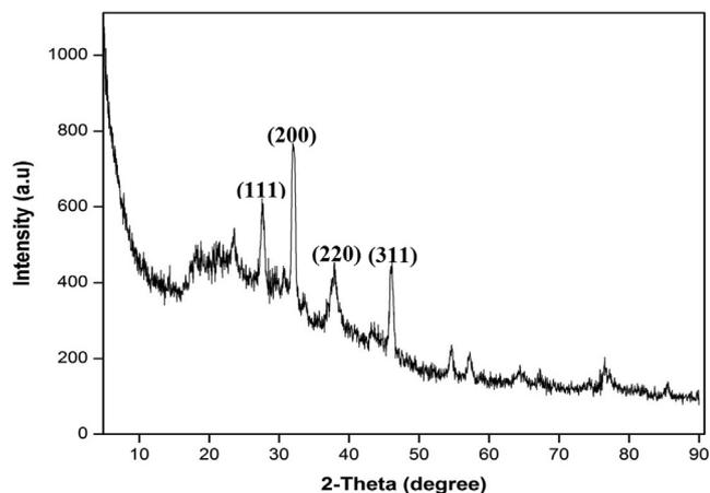
Fig 5. XRD spectrum of green synthesized silver nanoparticles.
