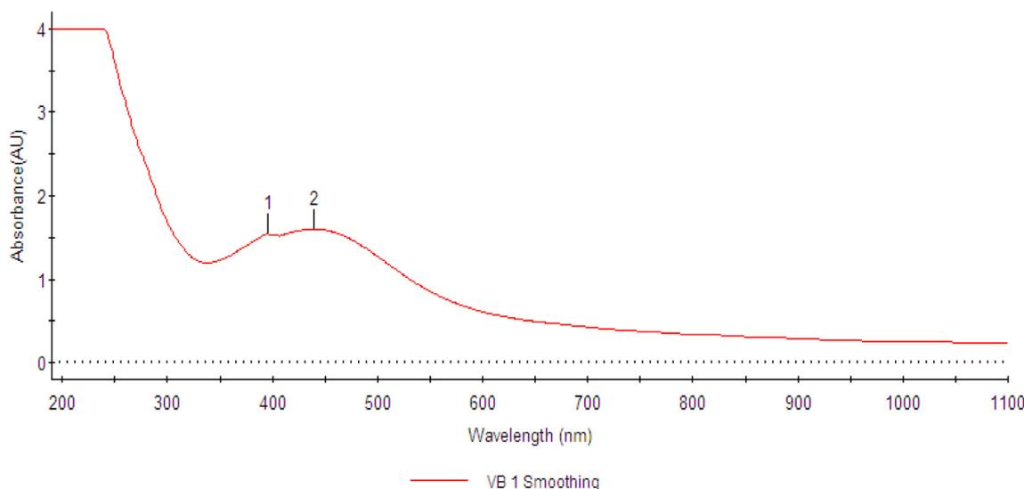
Fig 2. UV-Vis absorption spectra of green synthesized AgNPs.
