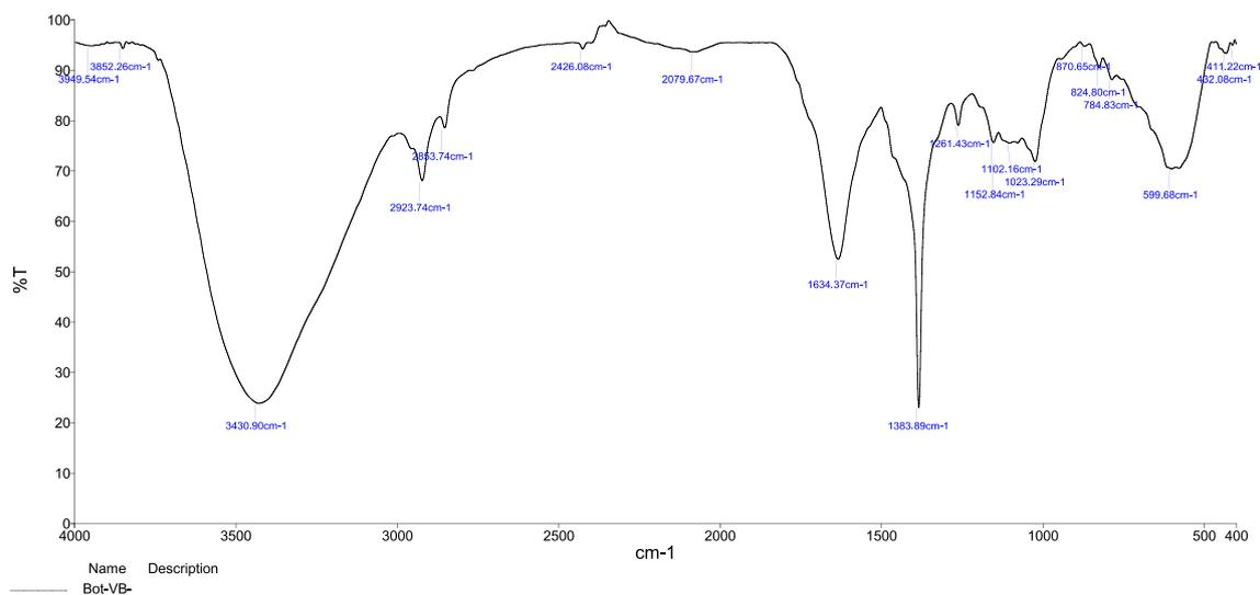
Fig 3. FTIR spectra of green synthesized AgNPs.
