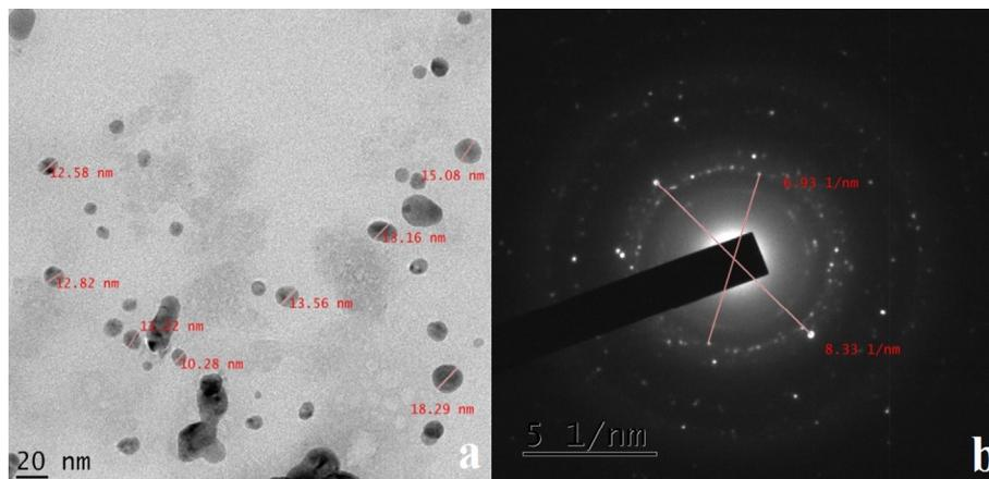
Fig 7. (a) TEM image of green synthesized AgNPs, and its SAED pattern (b) of green synthesized AgNPs.
