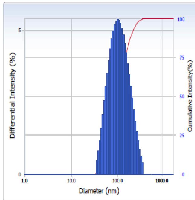
Fig 4. Dynamic Light Scattering (DLS) plot for green synthesized AgNPs.
