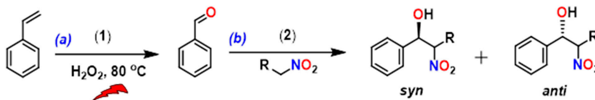
Scheme 2. (a) Microwave-assisted peroxidative oxidation of styrene to benzaldehyde catalyzed by trans -[CuL 2 (H 2 O) 2 ] ( 2 ); (b) Nitroaldol (Henry) coupling of benzaldehyde with nitroalkanes (R = H or Me) catalyzed by cis -[ZnL 2 (H 2 O) 2 ] ( 1 ).
