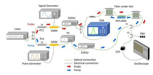
Figure 5. Experimental BOTDA setup.
