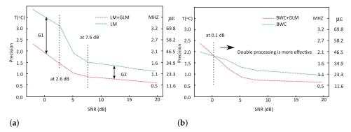
Figure 8. Measurement precision demonstrated by studied methods: (a) LM; (b) BWC.
