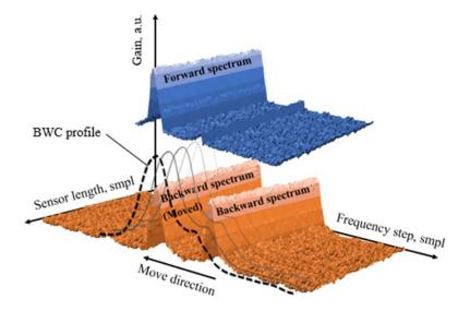
**Figure 2.** A schematic diagram combined using real data, describing the method operation principle (blue graph—forward spectrum; orange graph—backward spectrum with its shifted copy; dotted line—backward correlation function).
