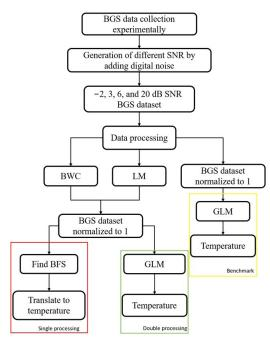
Figure 6. Data processing principle.
