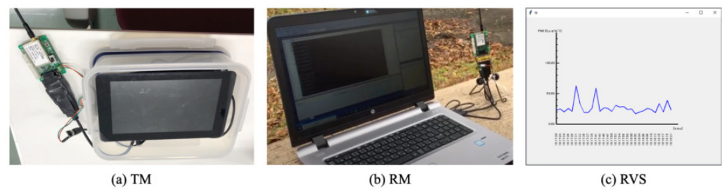
Figure 5. Assembled transmitter module (TM) and receiver module (RM) consisting of LCS.
