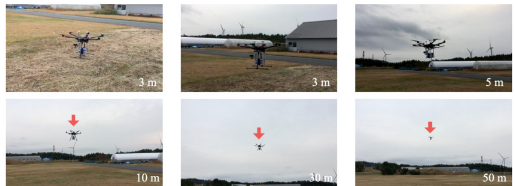
Figure 20. Photograph of D2 flight experiment. The numbers in the lower right corner of respective photographs indicate the approximate distances between the photographer and the drone.
