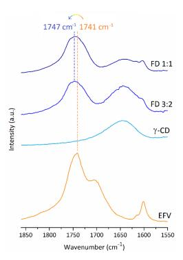
**Figure 3.** Fourier-transform infrared spectra of efavirenz (EFV),  $\gamma$ -CD and the two freeze-dried solid products starting from mixed solutions with  $\gamma$ -CD:EFV proportions of 3:2 and 1:1 (FD).
