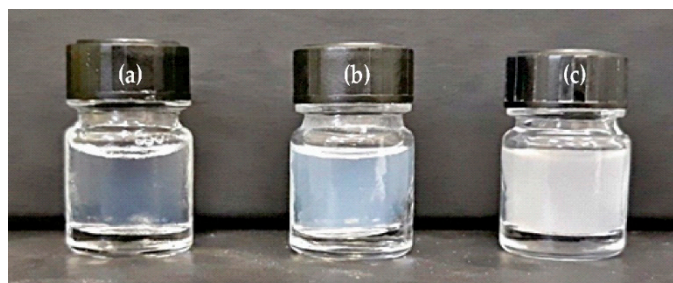
Figure 11. Visual aspects of the micellar solution of the PNVC-b-PCL (1) block copolymer ( C = 0.5 \text{ mg mL}^{-1} ) at different temperatures, at around: (a) 19 \text{ }^{\circ}\text{C} , (b) 29 \text{ }^{\circ}\text{C} and (c) 40 \text{ }^{\circ}\text{C} .
