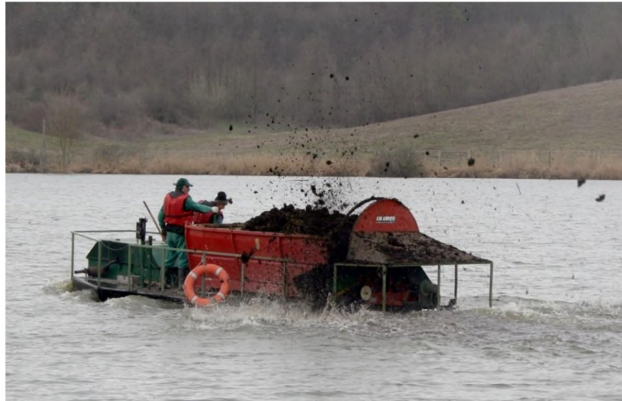
Figure 37. Specifically constructed shredding equipment, the so-called “manure-spraying machine”, helps to cut the large particles of manure into smaller ones, thus increasing the surface for a fast bacterial decomposition. Some of the small organic particles (detritus) are directly utilized as food by members of the zooplankton and zoobenthos.
