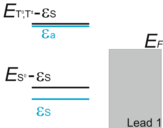
Figure 4. Scheme of the energy levels illustrating filling of the singlet S^0 state.
