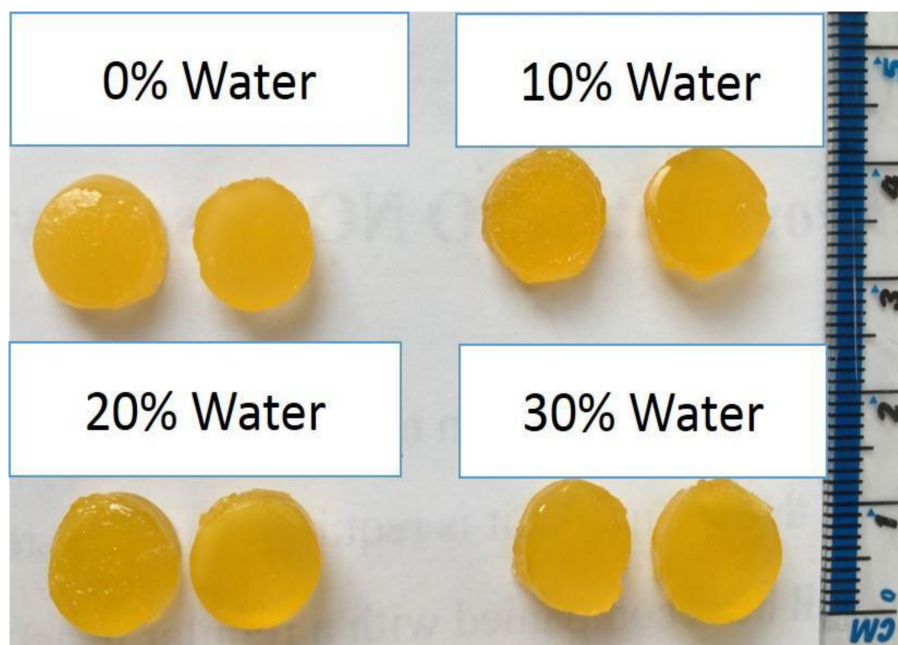
Figure 12. Hydrogels printed with riboflavin/triethanolamine as the photoinitiator with various water contents.
