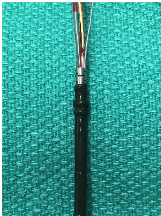
FIG. 4. Accordioning of the distal bending rubber component of the retained ureteroscope.
