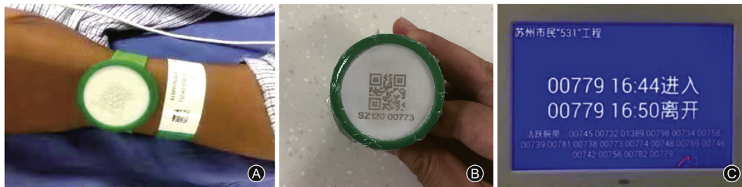
Fig. 1. Radio frequency identification devices (RFID) wristband is automatically record each key time point. (A) The RFID wristband is bound to the patient’s ID card information. (B) There is a QR code on the RFID wristband for quick identification by scanning the code. (C) In each link of the patient’s treatment, the RFID wristband automatically records the time and summarizes it into the Medicalsystem trauma system.
