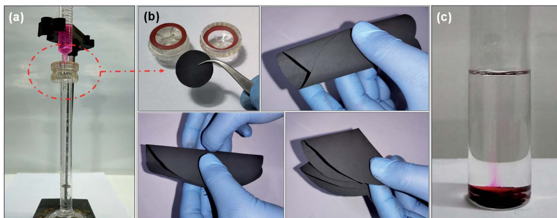
Fig. 7 (a) Digital image of the nano-filtration setup. (b) Digital image of the designed membrane reflecting its flexibility, scalability, and free-standing nature. (c) Digital image showing the contaminant extrusion from the membrane, and subsequently, the reuse of membrane as well as the contaminant separately.
