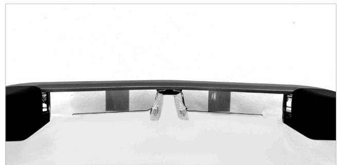
Fig. 1. The smart glasses (Moverio BT-300) from the wearer's perspective. Two OLED (organic light-emitting diode) lenses that display images are located at the center of the glasses.
