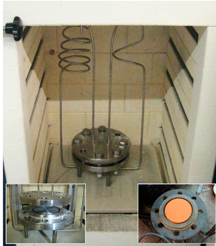
Figure 3. A prior version of the diffusion chamber mounted to the programmable lab kiln; insets show the opened chamber with spacer ring and steel dummy (left) or clay specimen (right).
