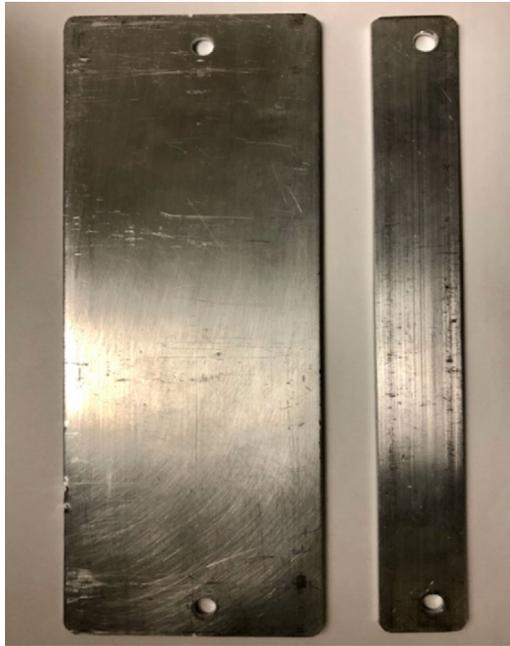
**FIGURE 1** An image of the fixed width (7.6 and 2.5 cm) of the individual aluminum bars that make up the compensator. These bars are all 21.8 cm in length. The holes are offset to the right of the middle of these bars to produce a tongue and groove effect when assembled
