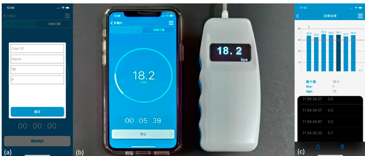
Figure 3. Screens of a novel tongue pressure measurement instrument: (a) measurement settings; (b) measurement screen in the smartphone and device; (c) results display screen.
