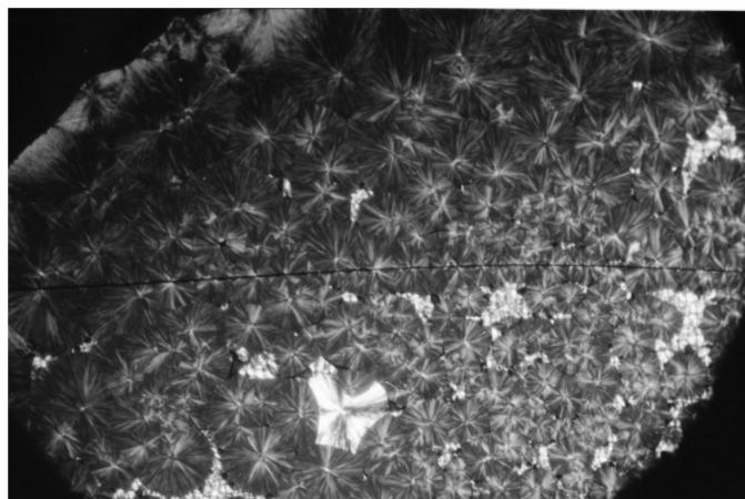
Figure 9. Differences in nucleation density of spherulites amongst regions within a specimen of iPP crossed by a carbon fiber.
