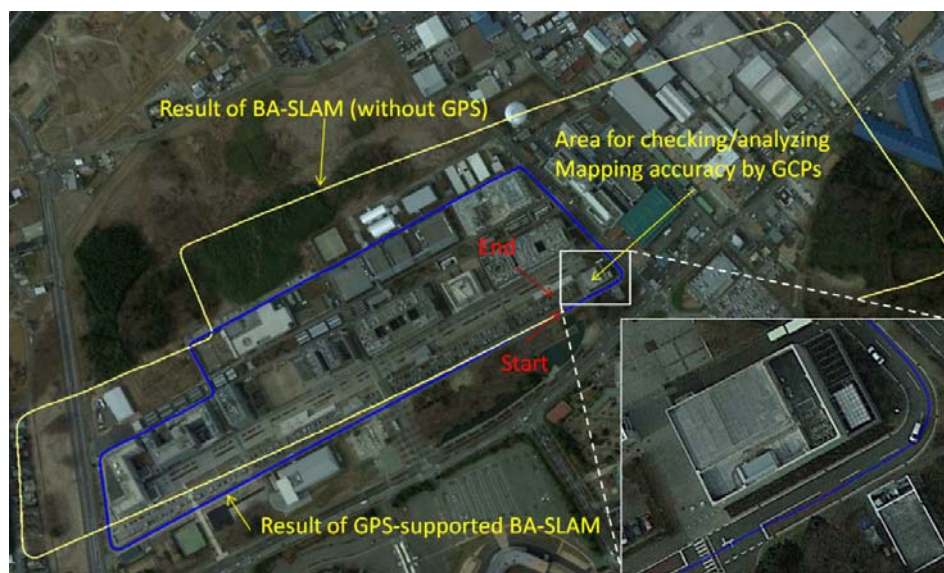
Figure 6. Results of the segmented BA-SLAM and GPS-supported BA-SLAM methods. The yellow line is the trajectory of the unconstrained results after data association and block BA. The start point is located in the correct position, but the trajectory shows a large accumulation of uncertainty in angle and scale. The blue line represents the trajectory after the GPS-supported BA-SLAM method is applied and shows a high level of accuracy. All eight GCPs are located in the enlarged area and are shown in Figure 7.
