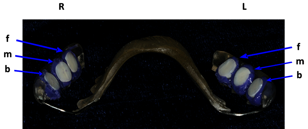
Fig 1. Individual upper jaw acrylic splint with six bovine enamel slabs (BES) embedded in silicon at different sites. The BES were fixed at the front (f), in the middle (m) and at the back (b), for both the right (R) and left (L) sides of the splint. Silicon covered the downward-facing surfaces and the margins of the BES and only their upward-facing surfaces exposed.
