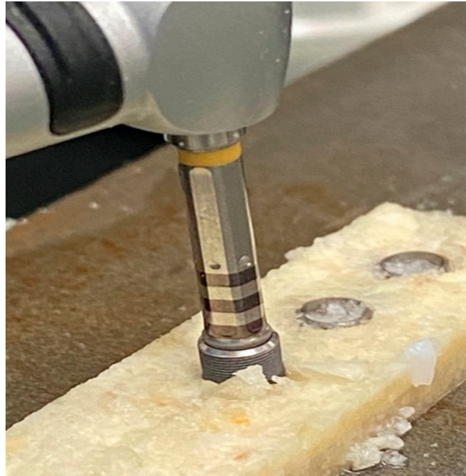
Figure 1. Implant insertion into junction of two artificial bovine bone plates held together by a vice.
