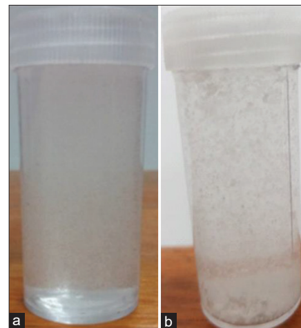
Figure 6: Appearances of the blood mimicking fluid sample in transparency glass. (a) After 3 weeks (1–6 weeks). A precipitate or float did not appear, and the acoustical properties didn't change. (b) After 7 weeks. The poly (4-methyl styrene) particles were started clotting, but precipitate or float did not appear too. Liquid density: 1.04 g/ml. Particle diameter: 3–8 \mu\text{m}
