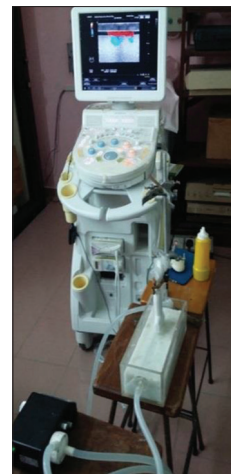
Figure 4: Vascular wall-less flow phantom construction using the clinical ultrasound scanner (Hitachi Avious Vision) at the Department of Medical Physics and Radiation Science, School of Physics, University of Science, Malaysia
