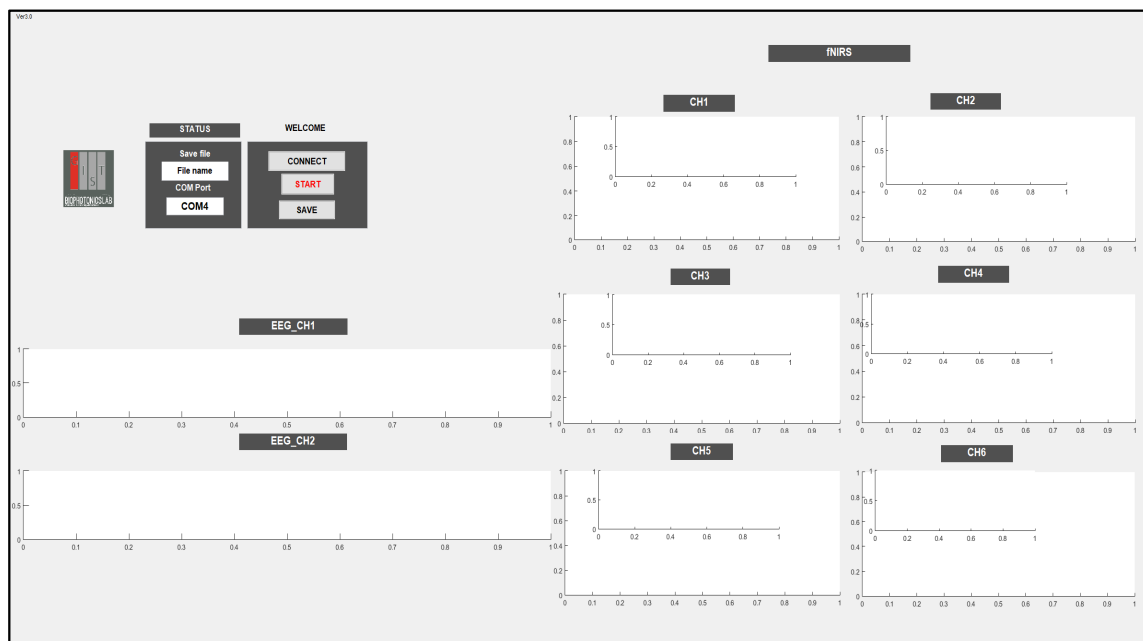
Figure 7. Graphical User Interface used to store and display EEG and fNIRS data.
