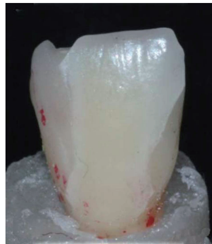
Fig. 6. An example of cohesive failure in laminates.
