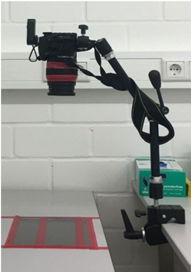
Fig. 1 Setting for measurement and for standardized digital image capturing
