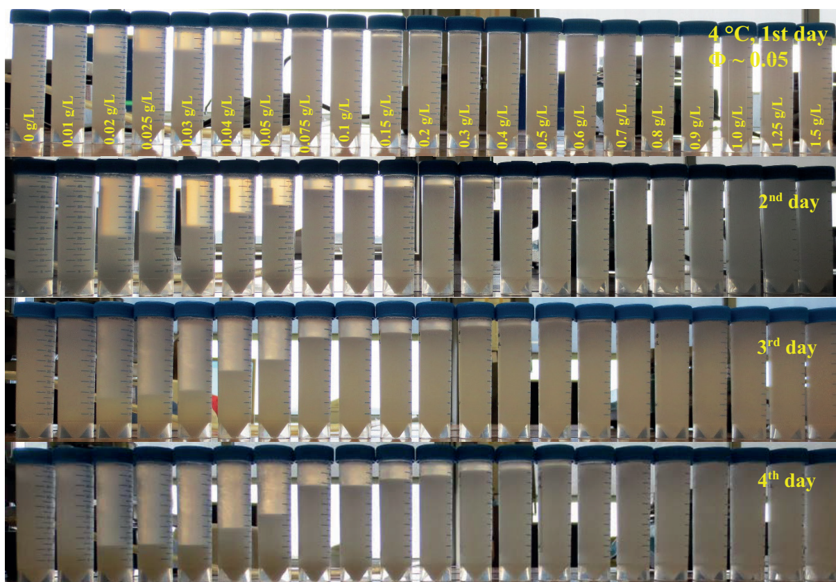
Figure 1. Pictures of WPI particle dispersions ( \Phi \sim 0.05 ) with different xanthan concentrations from 0 g/L to 1.5 g/L at 4 °C for 4 days.
