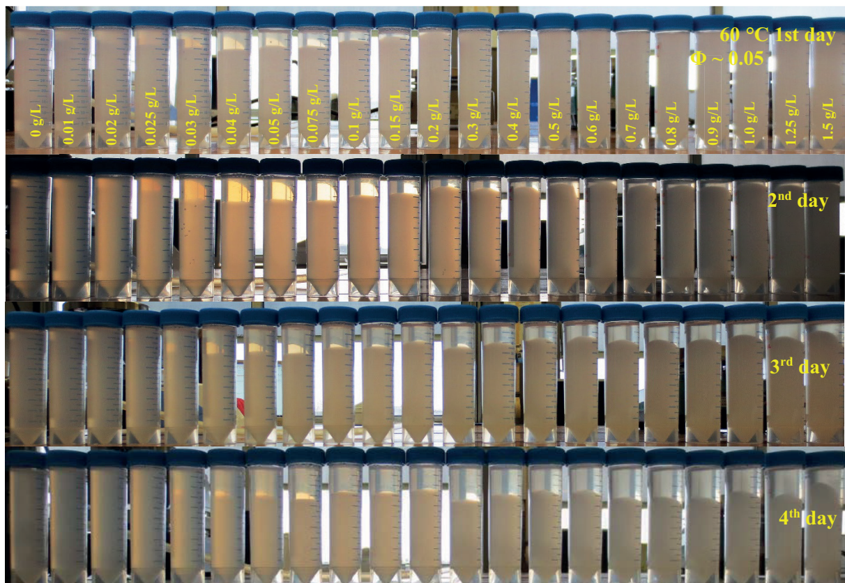
Figure 8. Pictures of WPI particle dispersions ( \Phi \sim 0.05 ) with different xanthan concentrations from 0 g/L to 1.5 g/L at 60 °C for 4 days.
