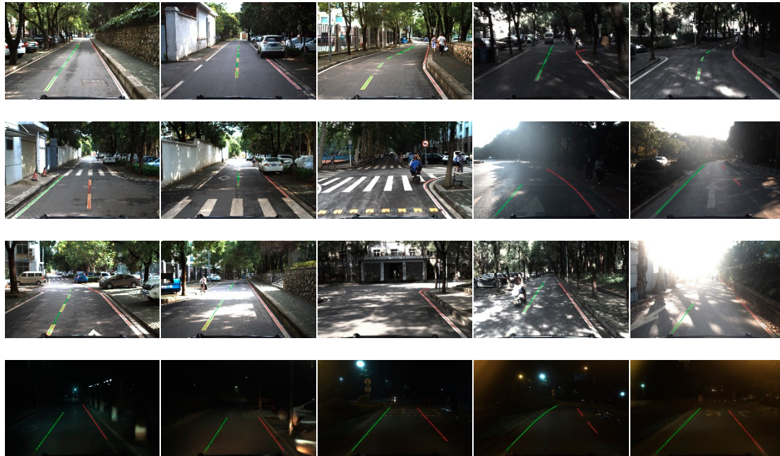
Figure 15. Some results of our method on a campus road, the left side of the current lane is colored with green and the right lane is red. The first row is in mild light conditions where the lane markings are constructed by straight line, polyline line or curb. The second row is in the intersections which contain zebra or arrow markings on the road. The third row was in bright light conditions which contain shadow, bright spot or backlighting. The last row consists of some night scenarios.
