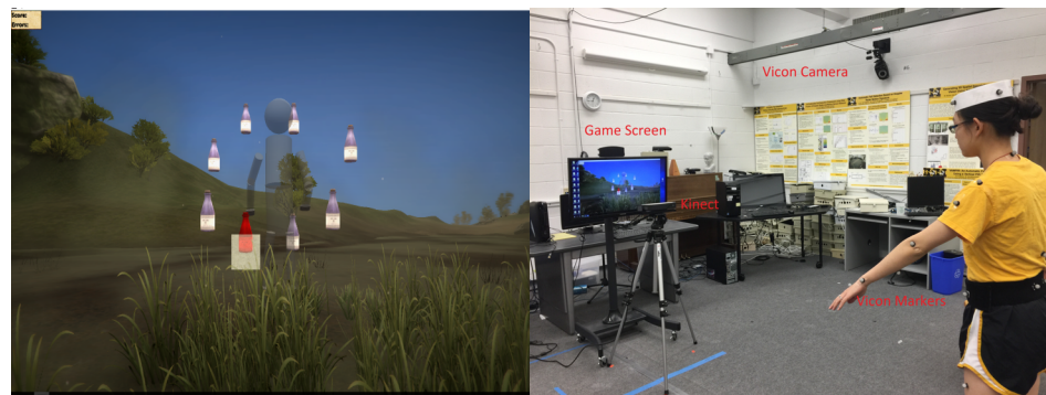
Fig 1. Mystic Isle game environment. (a) A virtual avatar collecting targets in a Kinect-based rehabilitation game, Mystic Isle . (b) A participant playing the game with Vicon markers on the body. Joint data of game trials were recorded by a Kinect and the Vicon system for validation.
