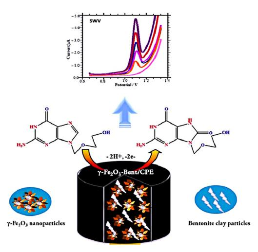
**Figure 5.** Schematic representation for the $\gamma$ -Fe<sub>2</sub>O<sub>3</sub>-Bent/CPE detecting ACV (reproduced with permission [6], copyright 2020, Elsevier B.V.).
