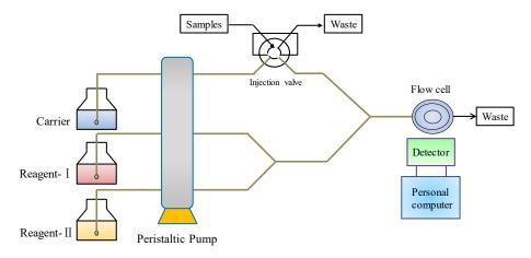
Figure 7. Schematic diagram of FI–CL analysis system.
