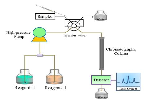
Figure 4. Schematic diagram of HPLC analysis system.
