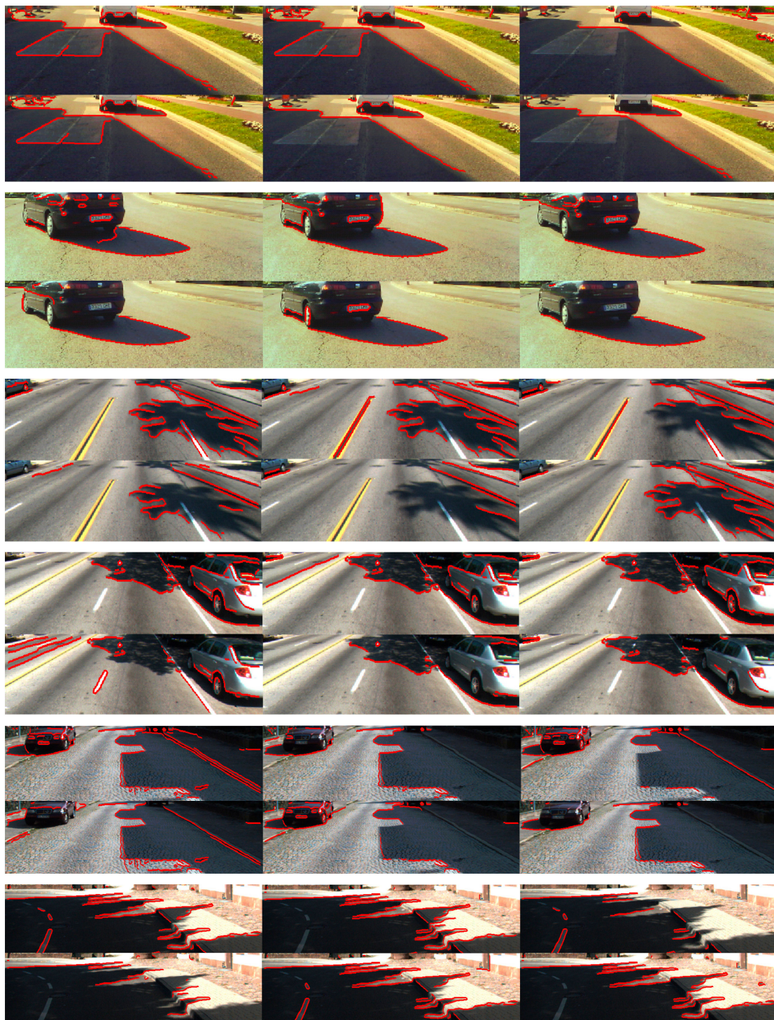
Figure 22. Shadow edge detection results obtained using the five methods. (First and second scenes) ROI of images of our dataset; (third and fourth scenes) ROI of images of the Caltech Lane dataset; (fifth and sixth scenes) ROI of images of the Kitti Road dataset. For each scene: Top-left results of Method 1; top-center results of Method 2; top-right results of Method 3; bottom-left results of Method 4; bottom-center results of Method 5; bottom-right results of our method.
