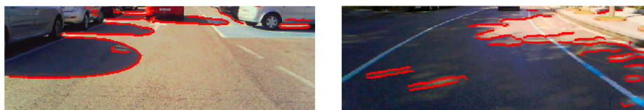
Figure 4. Shadow edge detection obtained by the three constraints in Property 2.
