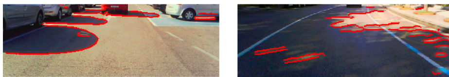
Figure 7. Shadow edge detection results obtained after applying the three properties all together.
