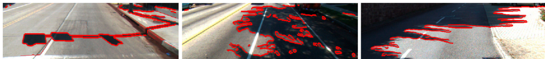
Figure 17. Shadow edge detection results of images in Figure 12 obtained by the proposed method.
