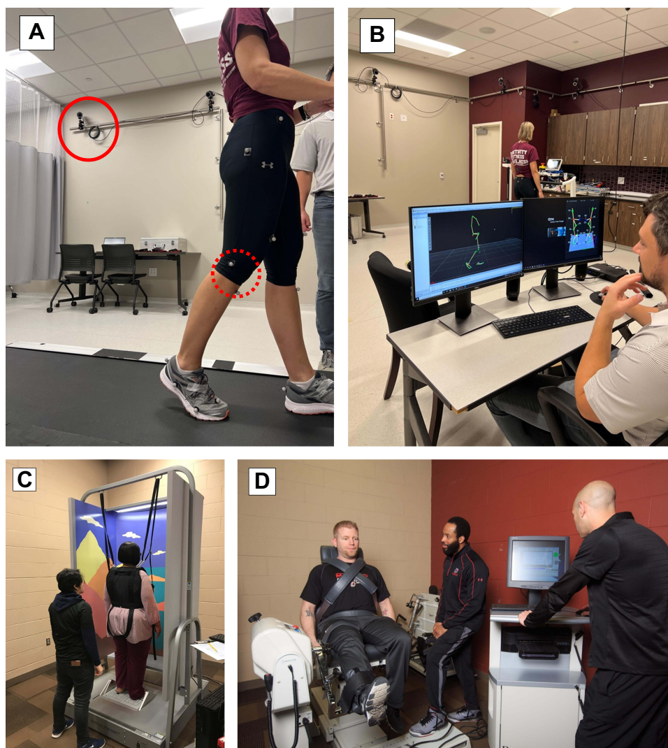
Figure 2 Typical biomechanical methods. (A and B) Motion capture represented by cameras systems in the background (solid red circle) record where markers are in space (dotted red circle) and provide information about where the person is in space (kinematics). (C) Force platforms provide information about forces (kinetics). (D) Dynamometers provide information regarding muscle strength and power.
