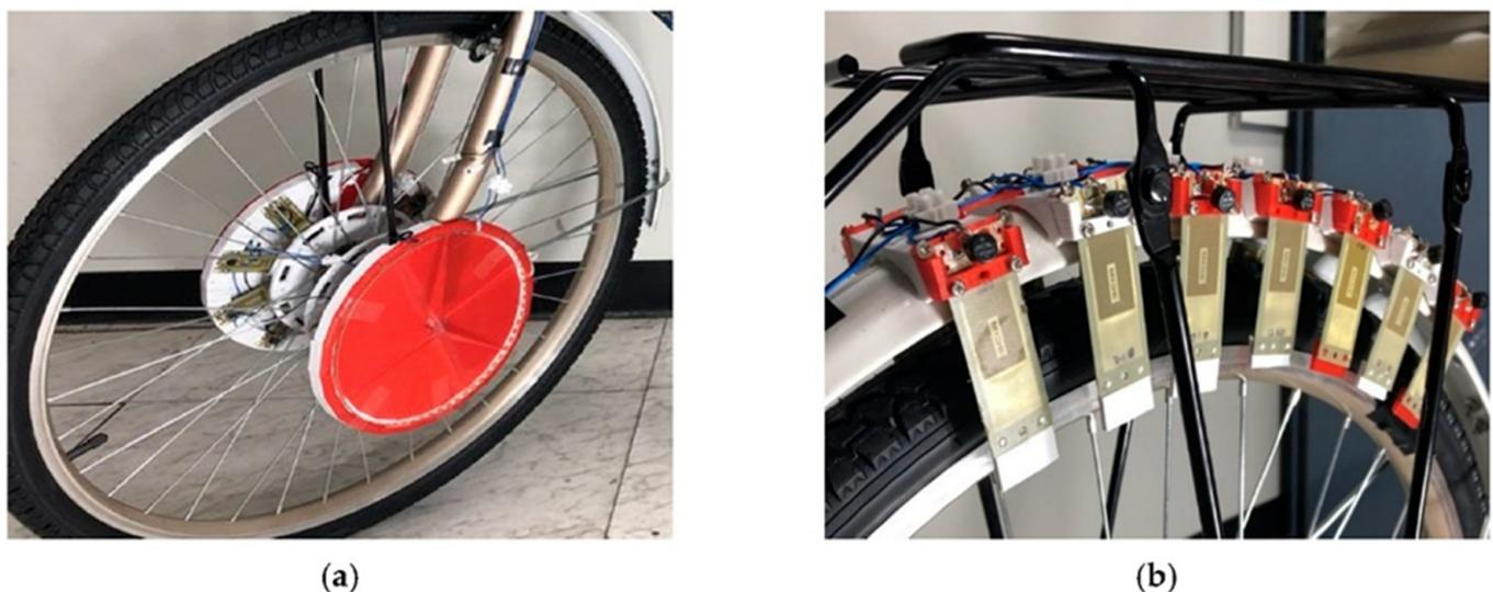
**Figure 5.** The installation of piezoelectric energy harvesters on a bicycle. (a) Piezoelectric harvesters installation distance at front wheel; (b) Piezoelectric harvesters installation distance at rear wheel fenders., adopted from [1].
