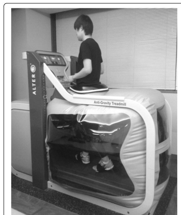
Fig. 1 Lower-body positive pressure (LBPP) treadmill. Participants walk on an LBPP treadmill. The positive pressure inflates the chamber to create traction force on the lower limbs
