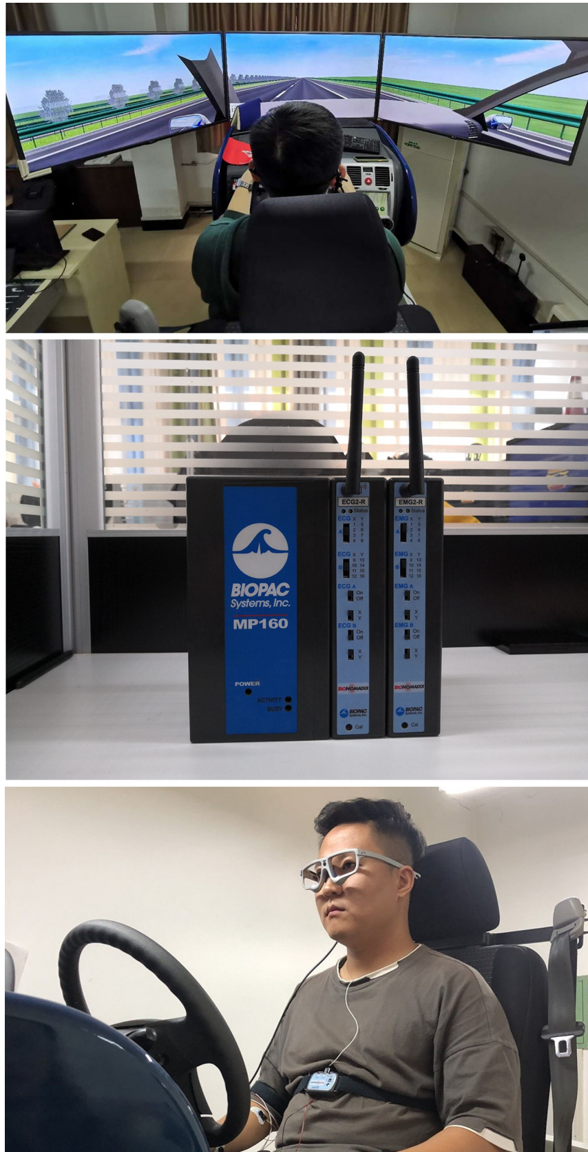
Fig 3. Experimental facilities. a) 6-DoF motion platform. b) MP150. c) SMI wireless glasses.
