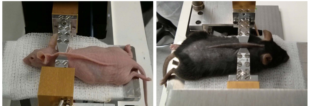
Figure 5. Images of the folded mouse back skin setting used to measure the transmittance of each sample for a diabetized nude (left) and a control black (right) mice.
