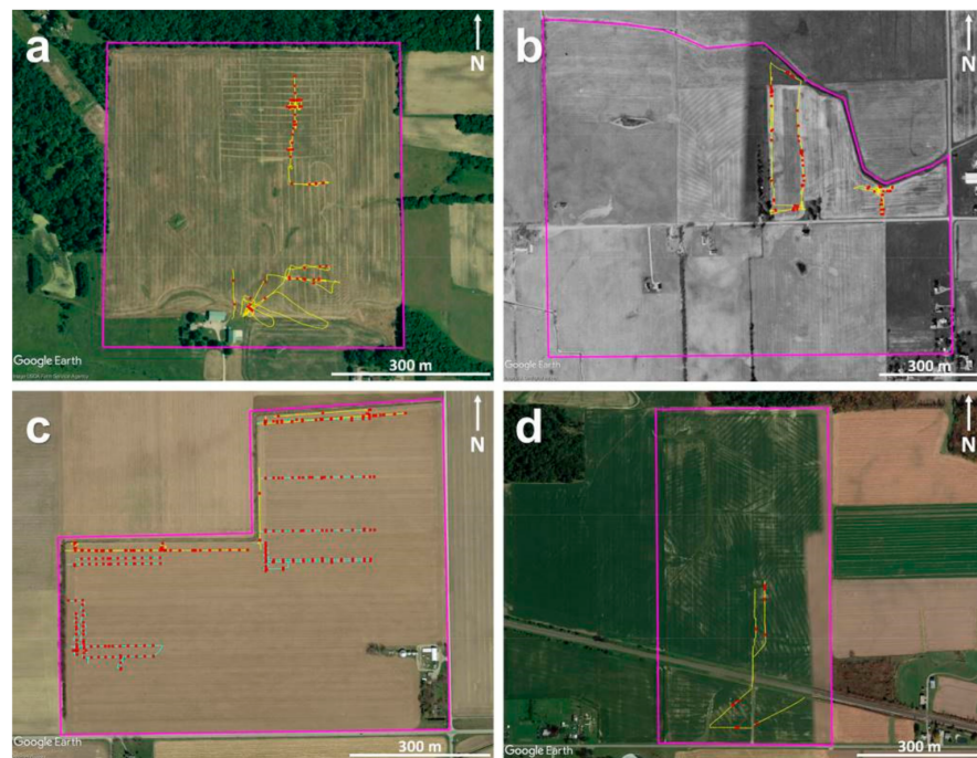
Figure 13. Potential drainage pipe locations marked (with red dots) on the GPR survey transects (yellow and cyan) overlaid on the Google Earth aerial images (same as in Figure 2): (a) Site-1, (b) Site-2, (c) Site-3, and (d) Site-4.
