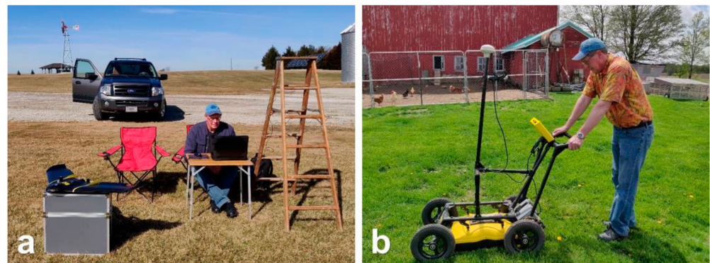
Figure 4. Equipment used in the investigation: (a) fixed-wing UAV, ladder with ground modem antenna, and computer, (b) SmartCart Noggin GPR system (250 MHz antennas).
