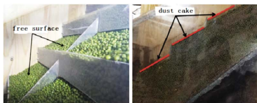
Fig. 4 The initial free surface and dust cake at the gas inlet.
