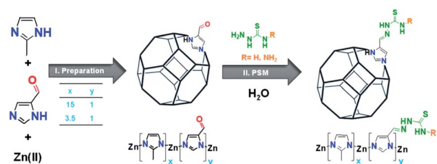
Scheme 1 Schematic illustration of (I) preparation of the two Ald-ZIFs (MIM x :AldIM y :Zn) and (II) post-synthetic modification (PSM) of Ald-ZIFs to obtain TSC-ZIFs through the incorporation of thiosemicarbazone derivatives (bisthiosemicarbazone and/or thiosemicarbazone) in aqueous solution.
