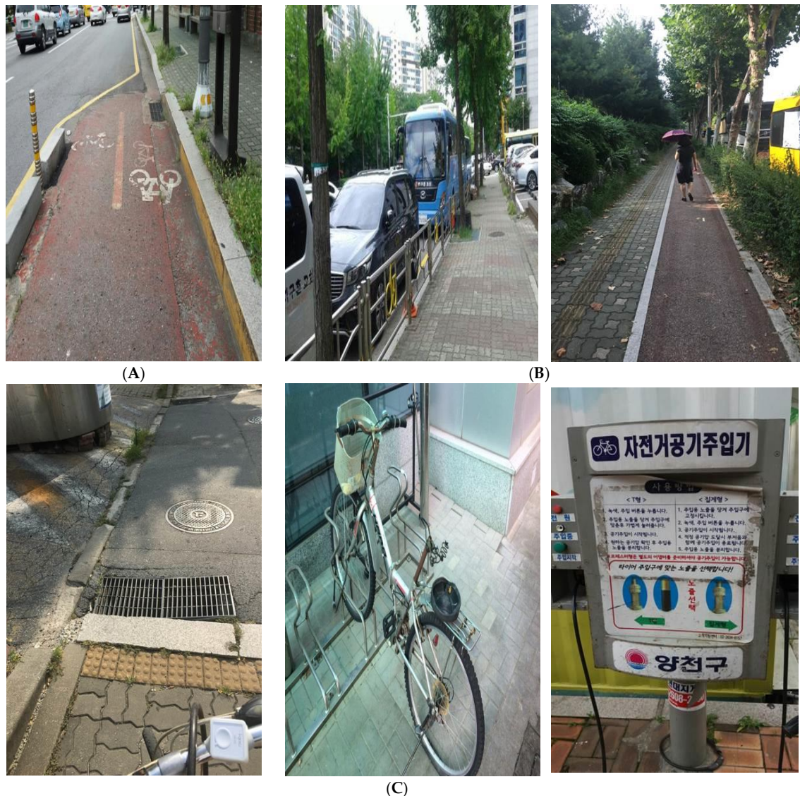
Figure 3. Factors that hinder bikeability. (A) “Bicycle-friendly” physical environment—Disconnection of cycle tracks. (B) Conflicts over bicycle use: (left)—Illegal parking; (right)—Pedestrian walking on bikeway. (C) Supportive community system: (left)—Poor management of road; (center)—A bicycle with a saddle stolen; (right)—Bicycle management equipment with insufficient instruction.
