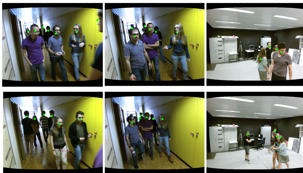
Figure 8. Detection results obtained under conditions of frequent occlusion, where the green points are the center points of the predicted bounding boxes.
