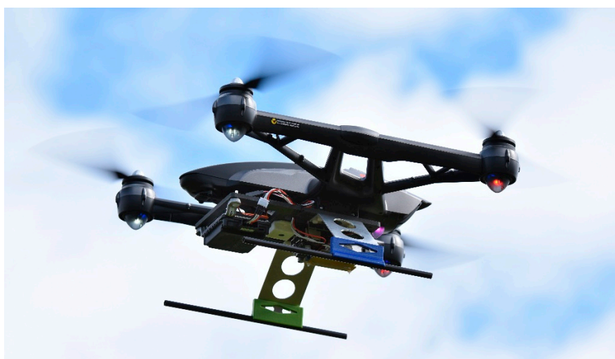
Figure 5. Test flight to check the measurement system with radar sensor ARS-404.
