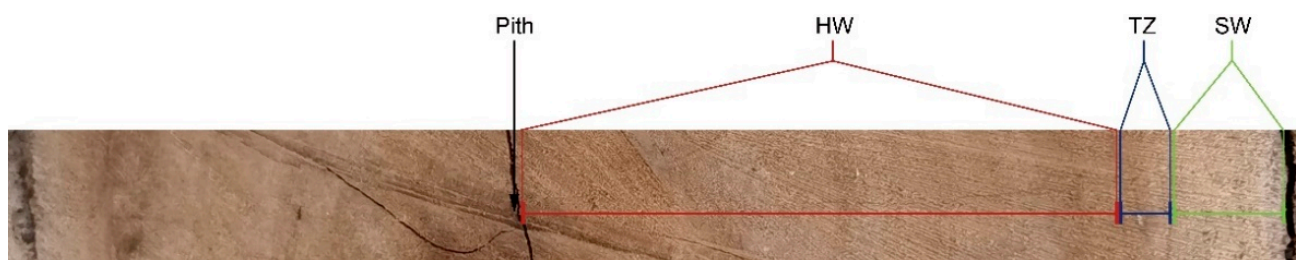
Figure 8. The sampling locations of different tissues of the P. hui wood strips. SW, sapwood; TZ, transition zone; and HW, heartwood.
