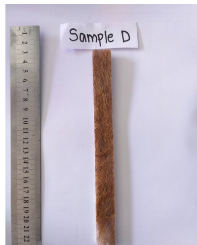
Figure 5. Specimen sample after cutting to 1.8 cm in width.
