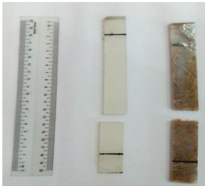
Figure 13. The sample of specimens after the tensile test.
