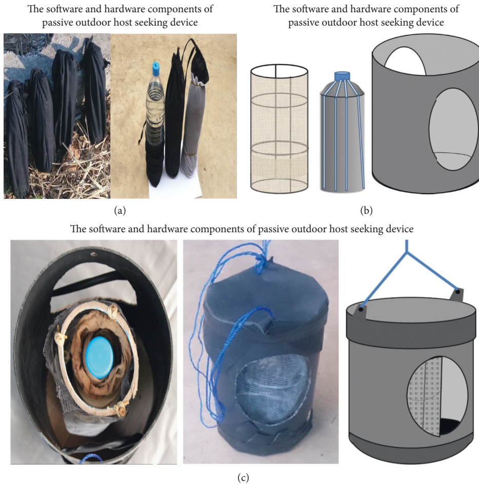
FIGURE 2: A prototype of a passive outdoor host seeking device (POHD). The designed POHD is made up of software and hardware components. The software components included (a) a bottle of water inside black cotton sack kept under solar power and (b) a bottle of water with nylon strips of attractants and a metal frame surrounded with electrostatic bendiocarb-treated or bendiocarb-untreated netting. The hardware component includes (c) the polyvinyl chloride (PVC) outer cover with two holes on sides, covered on top or bottom to protect the software components of the device.
