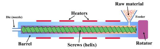
**Figure 2.** A simple schematic of extrusion processing, demonstrating the transformation of the raw ingredient (such as proteins and other reinforcement materials) to molded composites.
