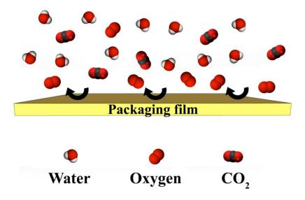
**Figure 3.** Schematic of barrier properties in packaging films against water, oxygen, and carbon dioxide molecules.
