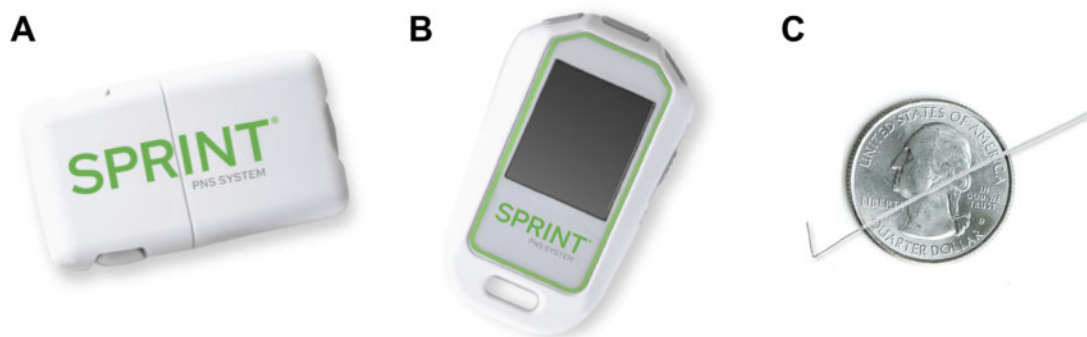
Figure 1. PNS system and lead. Participants received PNS via a rechargeable, body-worn stimulator (A), controllable by each patient by using a wireless handheld remote (B), delivered to the lumbar medial branch nerves through fine-wire, open-coil leads (C).
