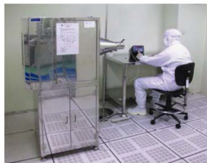
Fig. 2. Schematic diagram of Helmke Drum test method.
